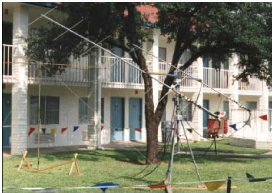
A portable antenna array for working OSCAR 10. The array consists of a 2-meter Yagi, a 70-cm Yagi, and an azimuth/elevation rotator.
